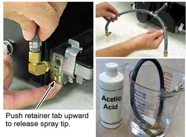
Push retainer tab upward to release spray tip.
