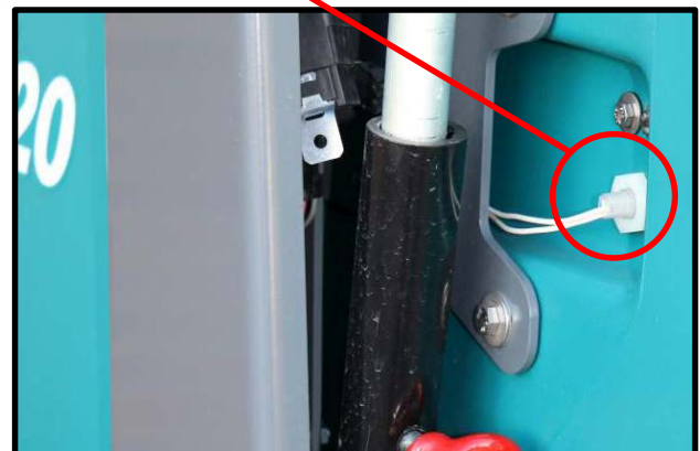
Recovery Tank Full Switch S-15
