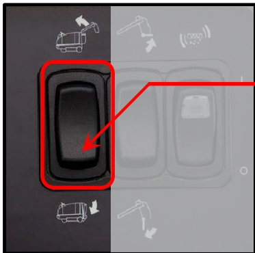
HOPPER LIFT/LOWER SWITCH PUSH TO LOWER HOPPER
