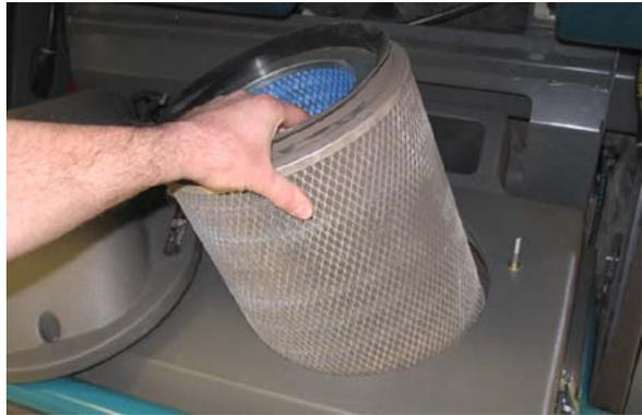
4. Clean or discard the dust filter element. Refer to *CLEANING THE DUST FILTER*.
