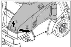
Note: The cover is equipped with a safety installation that switches off the drive when it is opened and issues a warning message on the display. If the cover is not properly closed the device will not operate.
