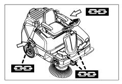
→ When transporting in vehicles, secure the appliance according to the guidelines from slipping and tipping over.
